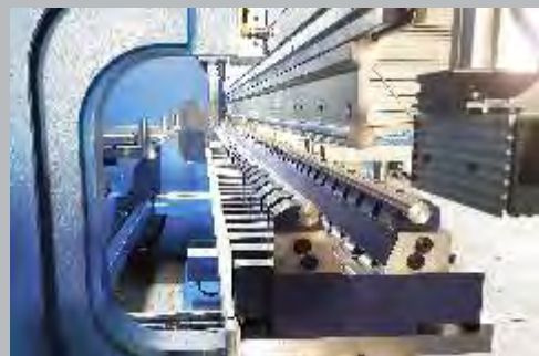
Special, heavy-duty, adjustable die, V=25 - 400mm
