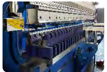
Adjustable Vdie system, CNC or manually adjusted (optional)
