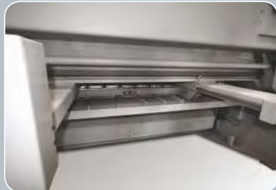
Position 1: Thanks to the RSS System, the sheet-metal is supported on the back gauge and does not bend.
