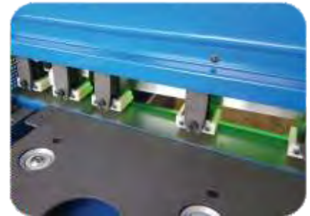
Specially-designed rectangular hold downs, suitable for cutting narrow stripes (optional)
