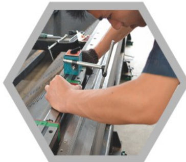
Parallelism Ball gear parallelism test
