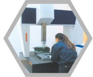
Precision 3 axes coordinate meter tests coordinate setting precision
