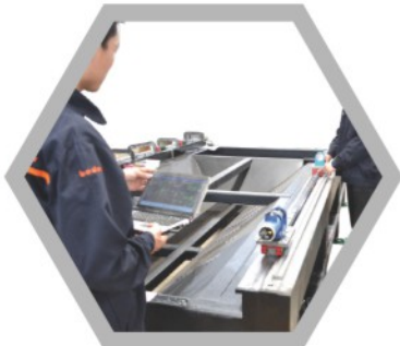
Straightness Laser collimator detects guide line
