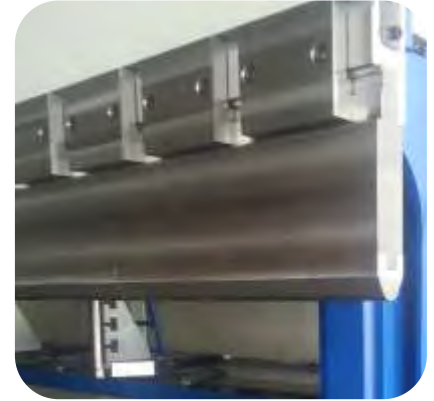
Heavy-duty clamping system up to 350t/m (optional)
