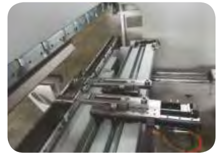
5-axis back gauge, X-X'-R-Z1-Z2 (optional)
