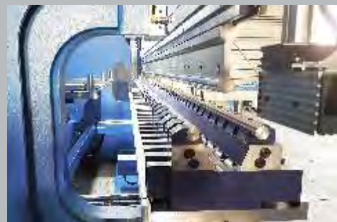
Special, heavy-duty, adjustable die, V=25 - 400mm
