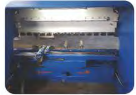
Back gauge guiding system on machine's sides (free space at the back)
