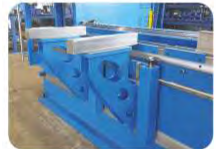
Heavy-duty front supports, moveable on linear guide, height adjustable (optional)
