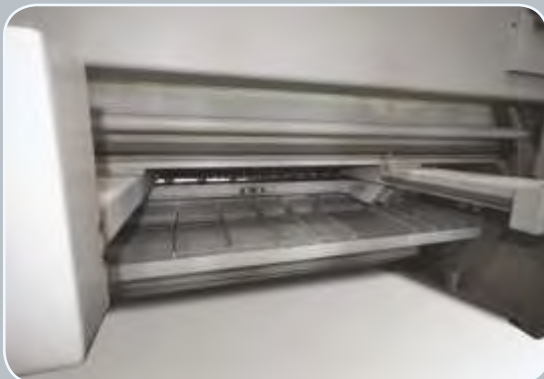
Position 2: The RSS moves downward about 150mm, stops and takes the entire sheet-metal to be cut so that the cut stripe does not bend due to its weight and touch the floor.
