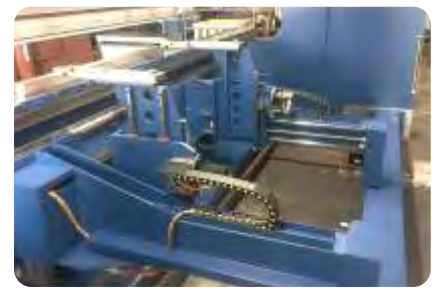
6-axis back gauge, X1-X2-R1-R2-Z1-Z2 (optional)
