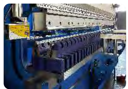
Adjustable Vdie system, CNC or manually adjusted (optional)
